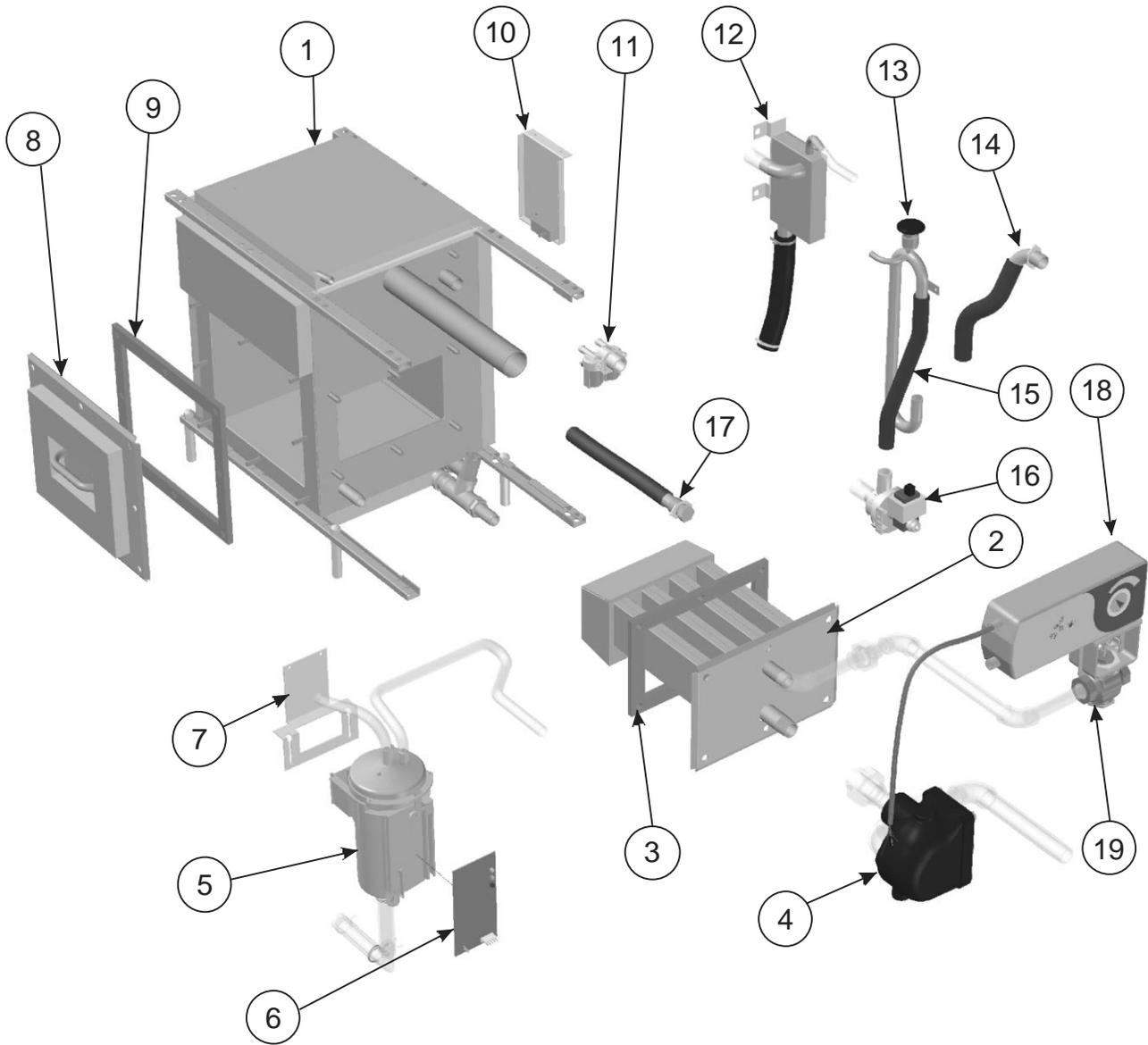
Figure 41: SETC 50 Plumbing Parts
