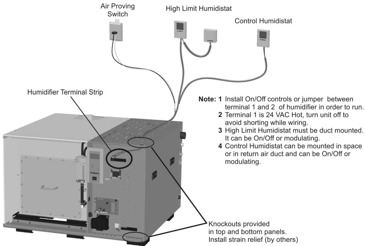
Figure 23: Dual Modulating Controls
