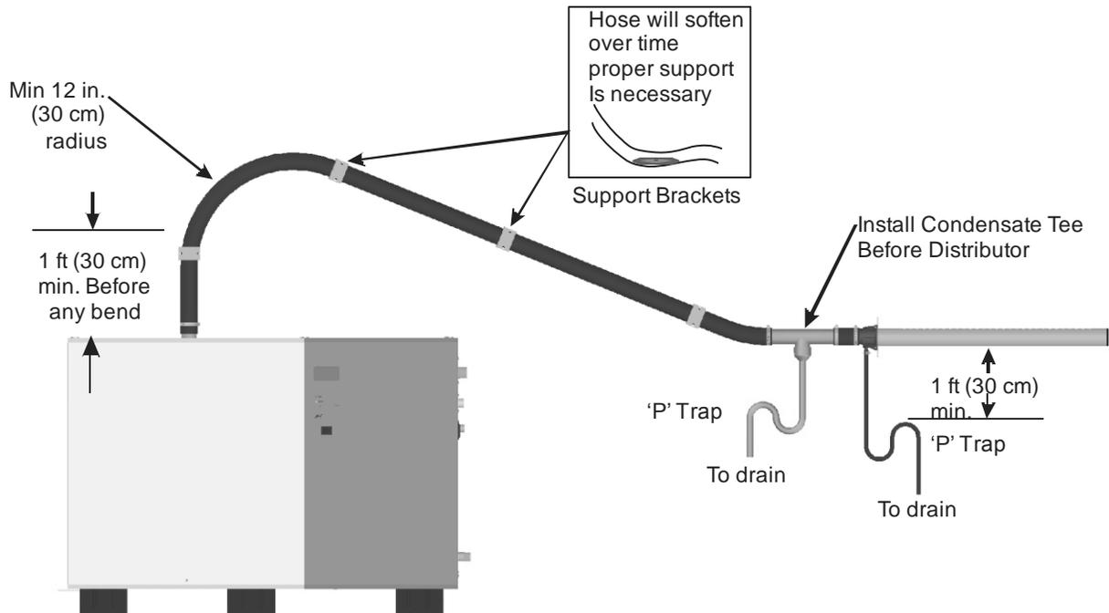
**Figure 17: Steam Distributor Below Humidifier (Hose Shown)**
