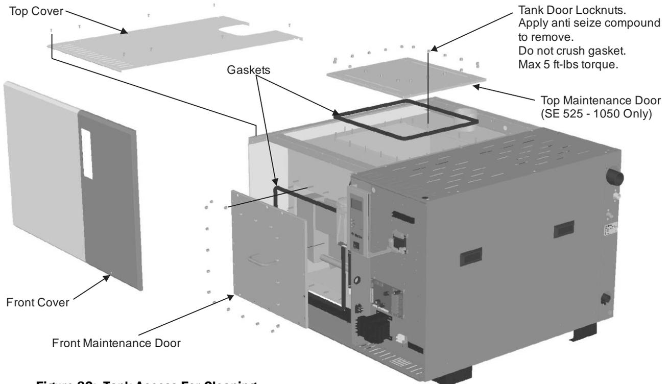
Figure 32: Tank Access For Cleaning
