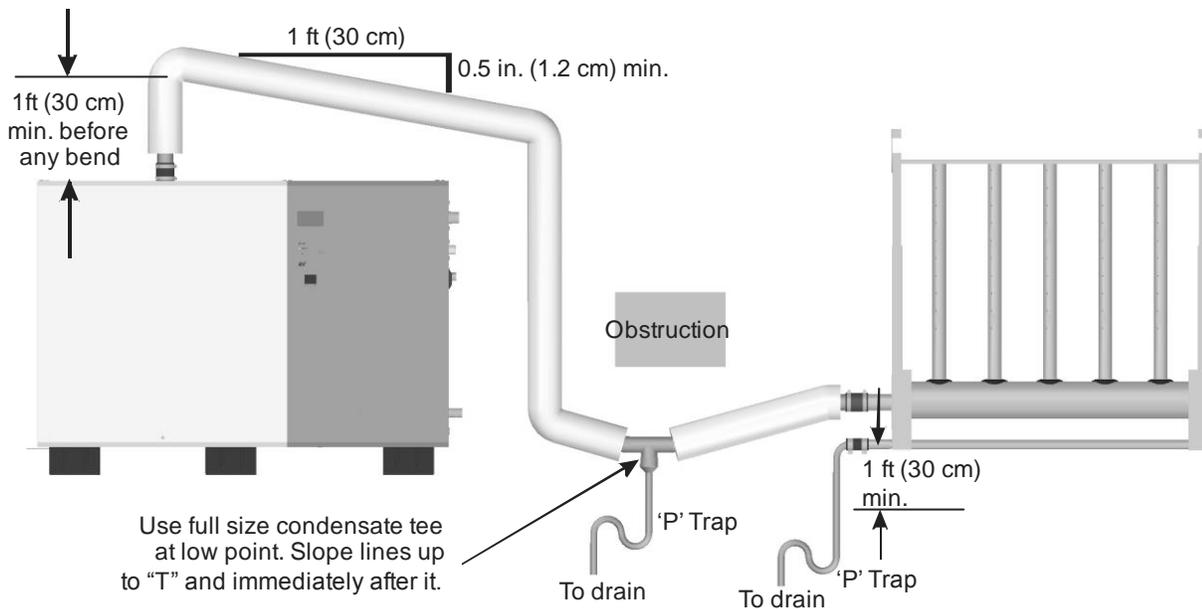
**Figure 18: Steam Under Obstruction (Copper Steam Line Shown)**
