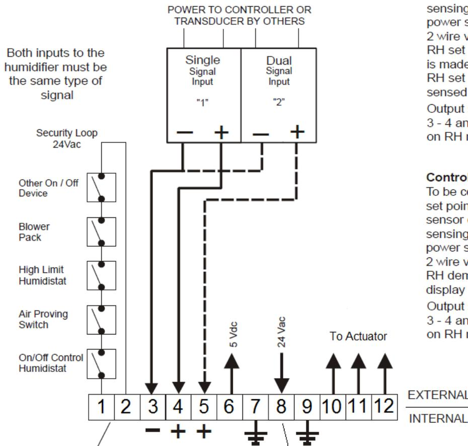
NOTE: If no On/Off Control is used then a field jumper must be connected across terminals 1 and 2 in order for the humidifier to operate.
