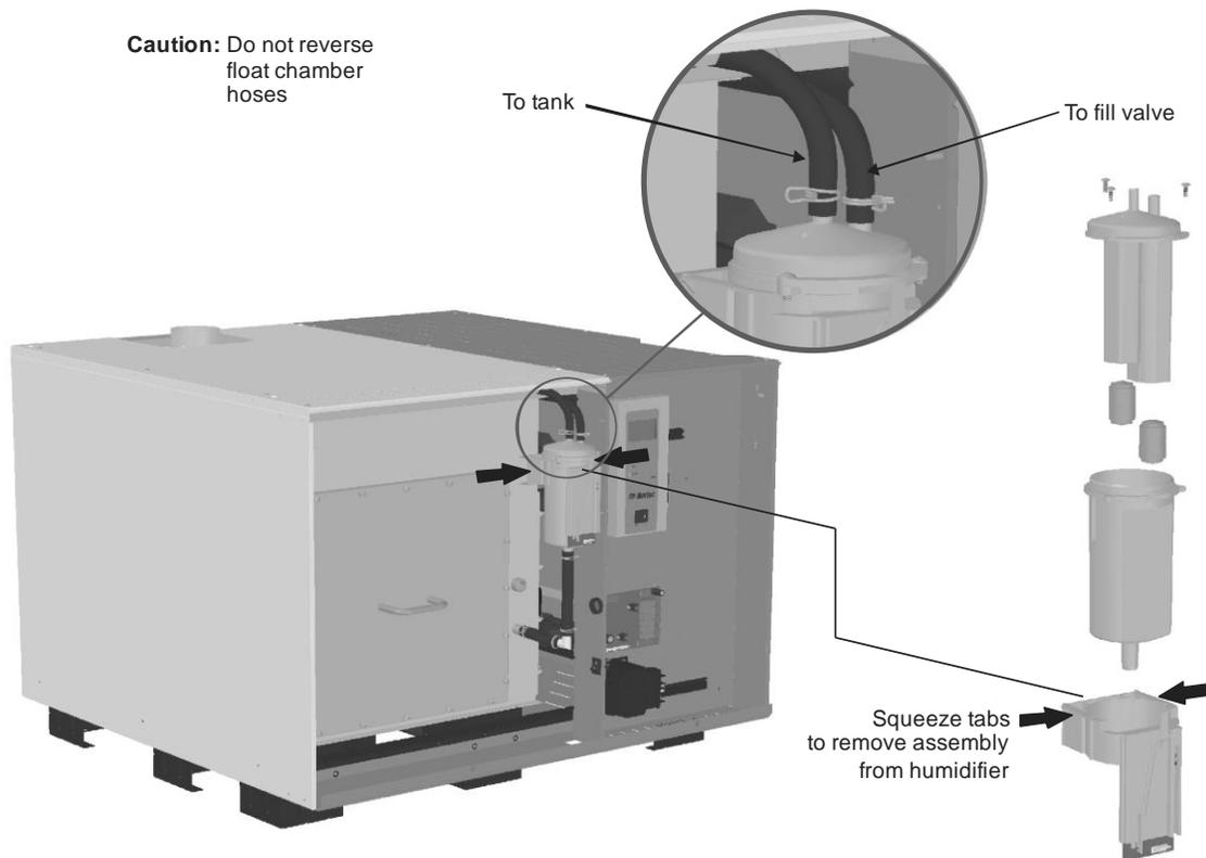
Figure 37: Float Chamber Cleaning
