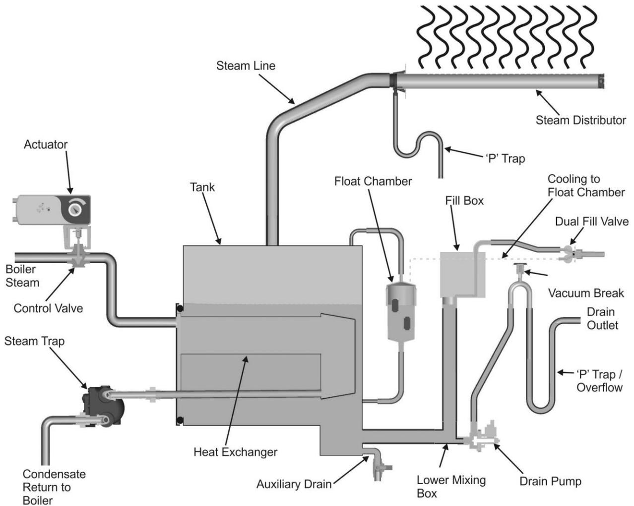
Figure 31: Humidifier Schematic
