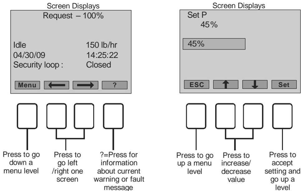
**Figure 33: Navigating the SETC Software**
