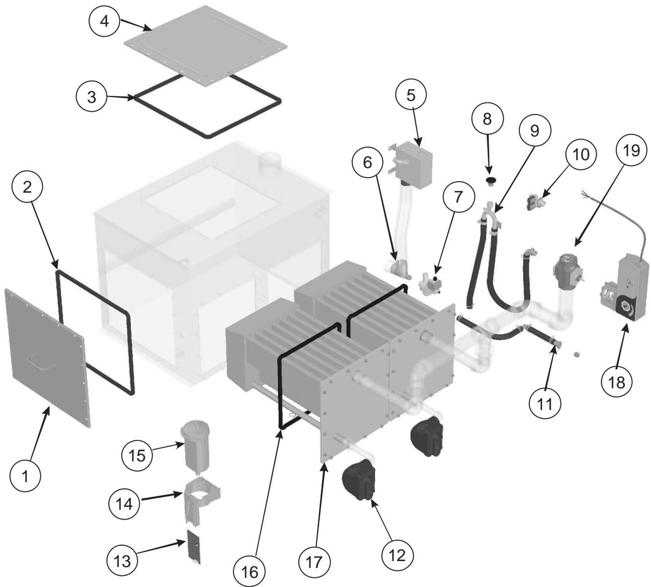
Figure 39: SETC 100-1050 Plumbing Parts
