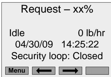
The LCD display will illuminate and the humidifier will perform a self-diagnostic sequence during which the LED's and internal components will be momentarily activated. The SE will then begin filling with water. The fill time is between 10 and 30 minutes depending on the size of the unit.
