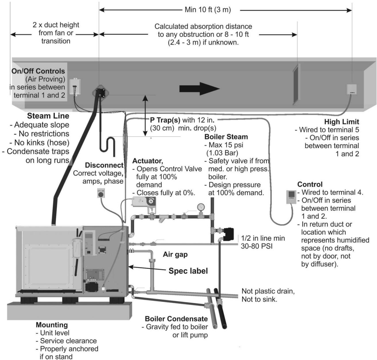
**Figure 27: Installation Check**
