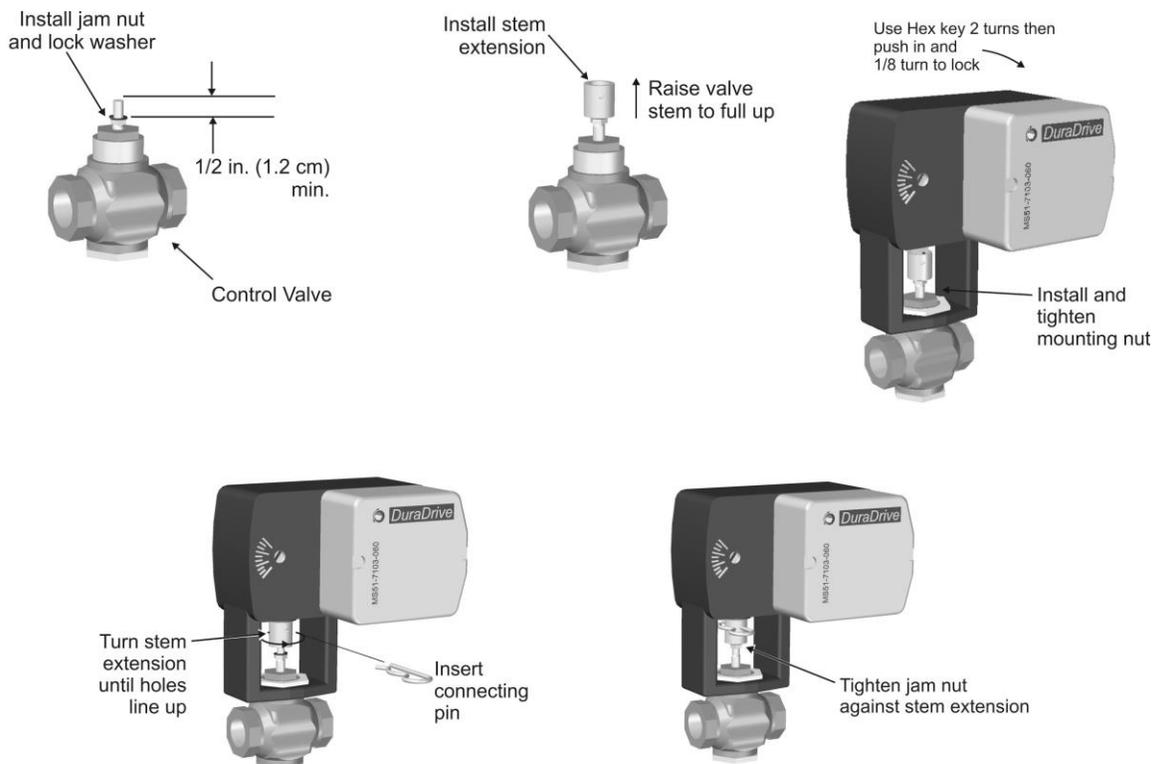
**Figure 12: Control Valve Actuator Installation**
