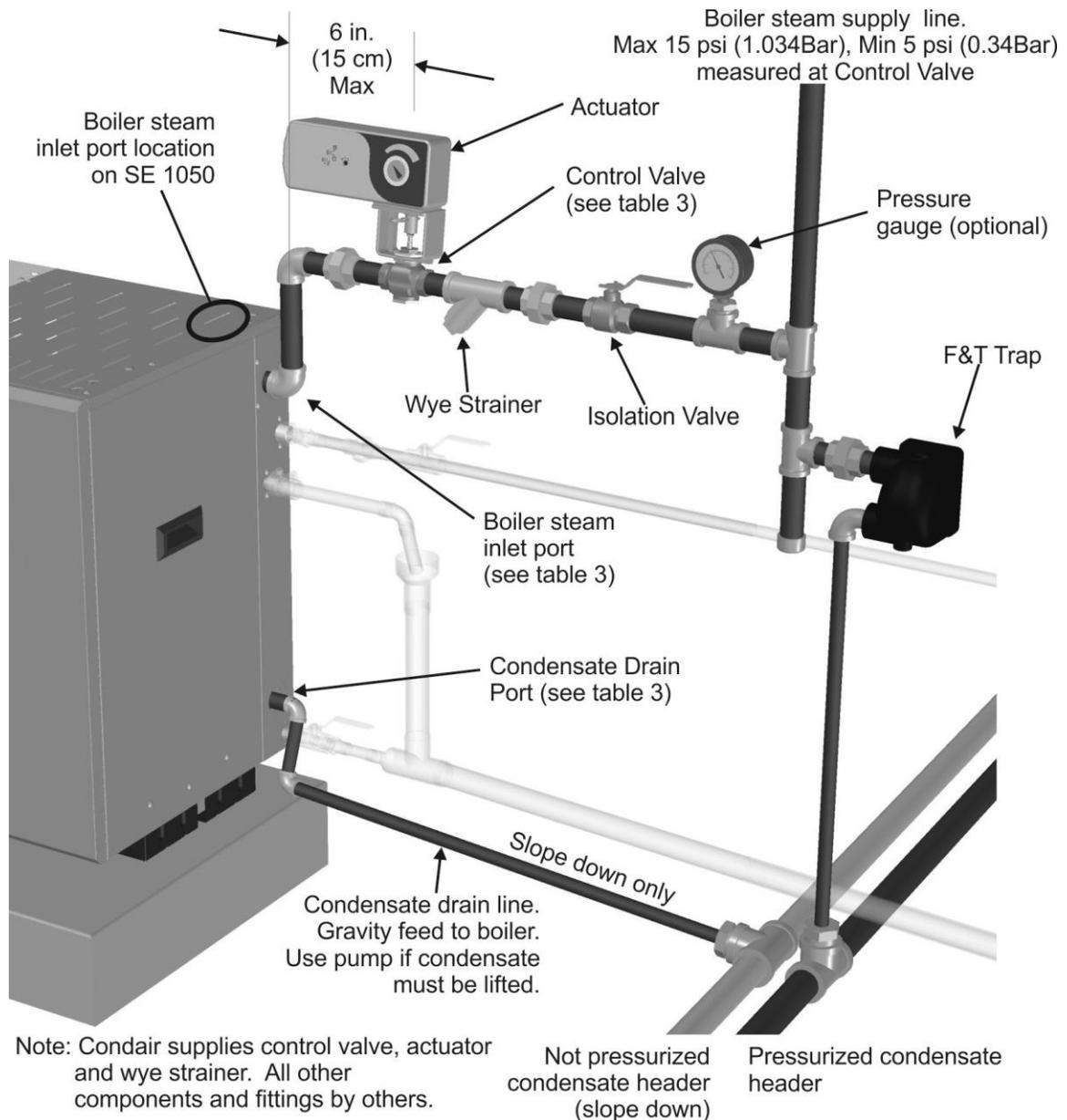
**Figure 11: SE Boiler Steam and Condensate Connection**
