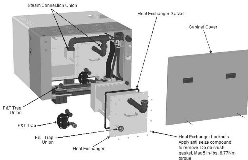
**Figure 336: Heat Exchanger Removal**
