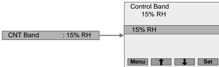
**CNT Band** should not normally be changed. The **CNT Band** setting adjusts the band within which the humidifier will modulate between 0 and 100% output. (Default = 15%)
