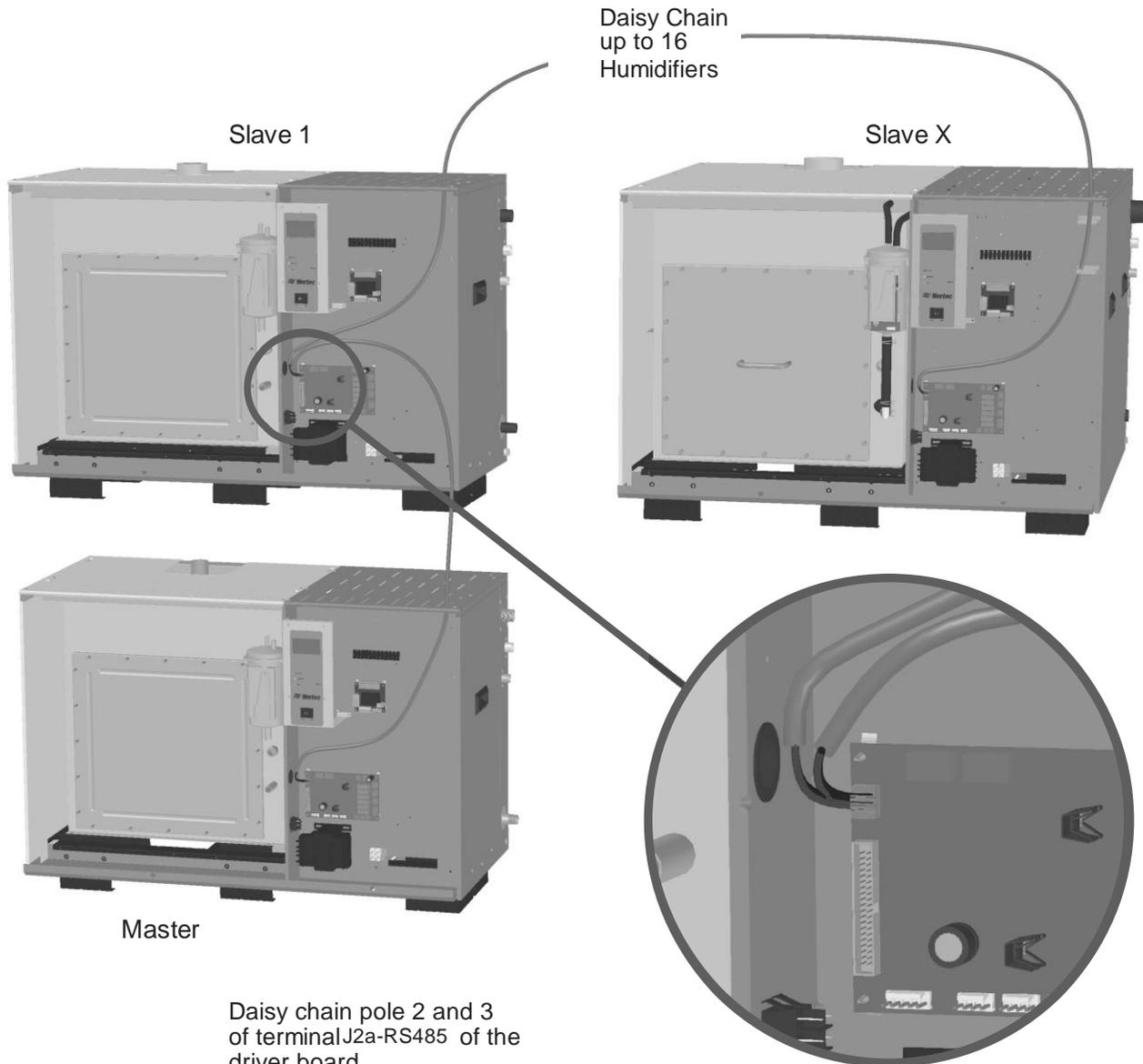
Daisy chain pole 2 and 3 of terminal J2a-RS485 of the driver board.
