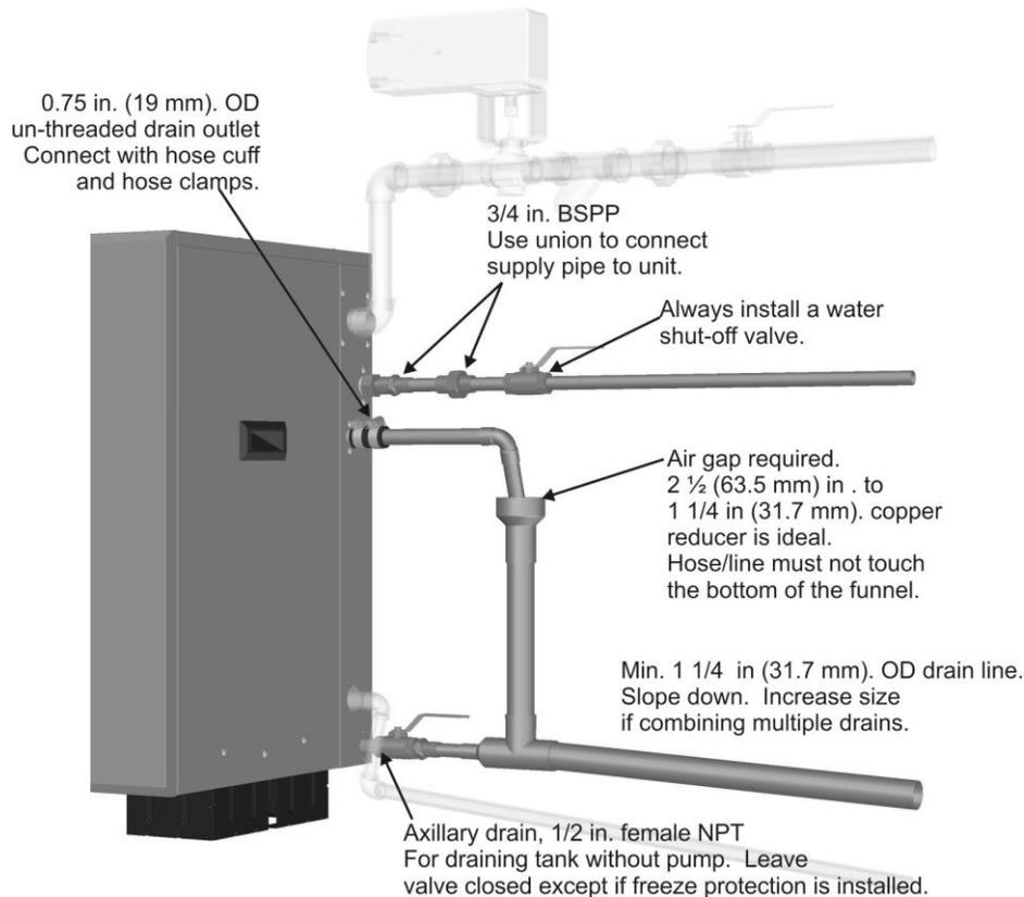
\*Pipe, unions, and water shut-off valve not supplied by CONDAIR.
