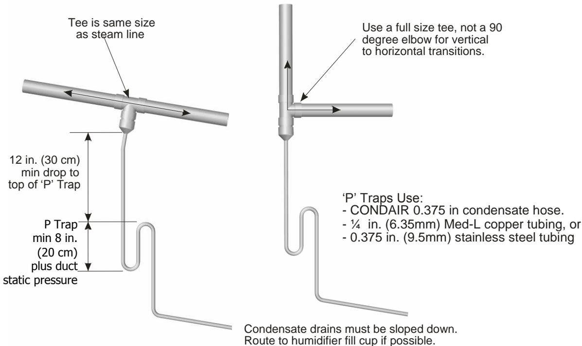
**Figure 14: Condensate Traps**
