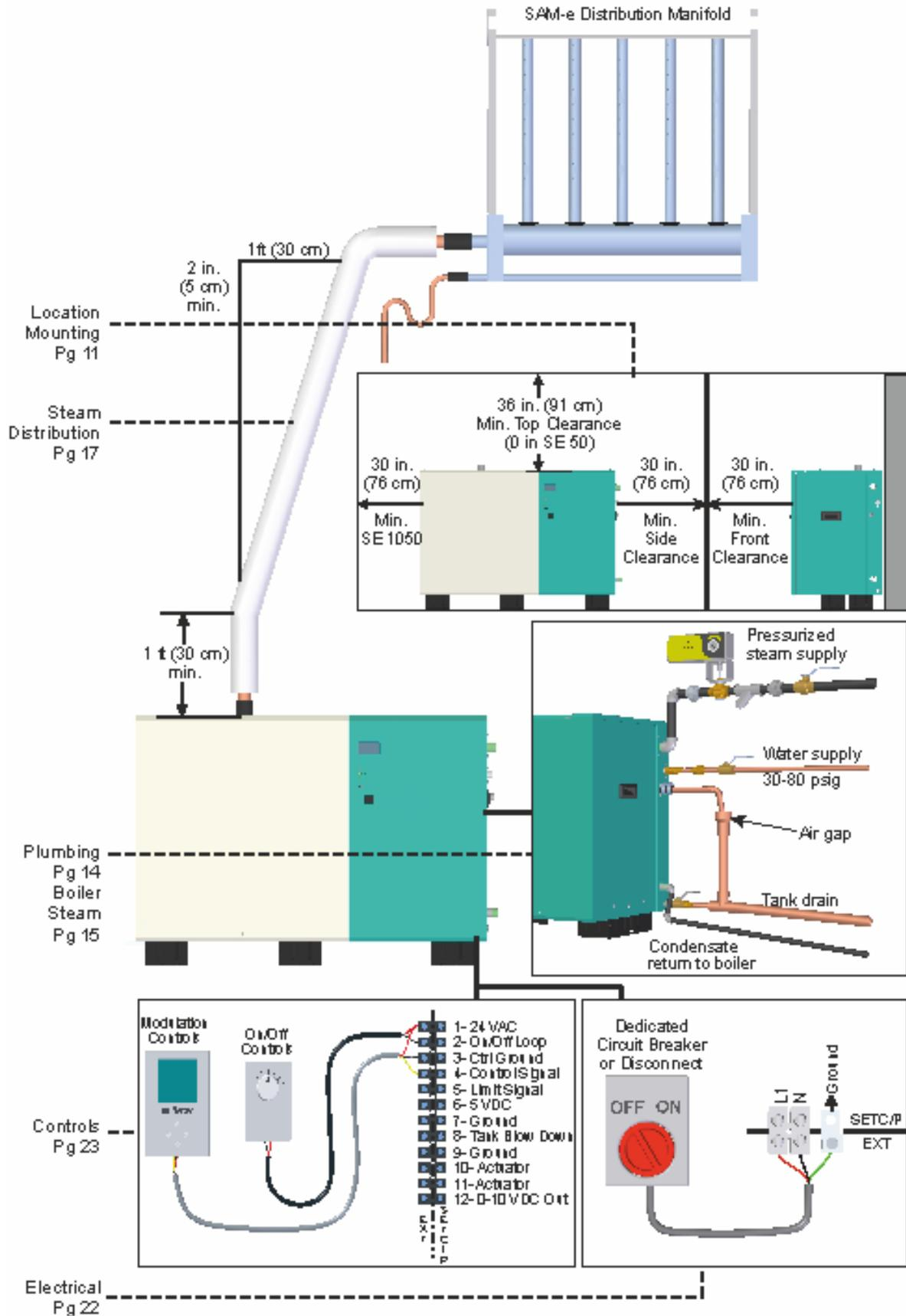
Figure 5: Typical Humidifier Installation
