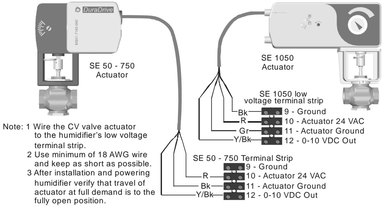
**Figure 24: Control Valve Actuator Wiring**
