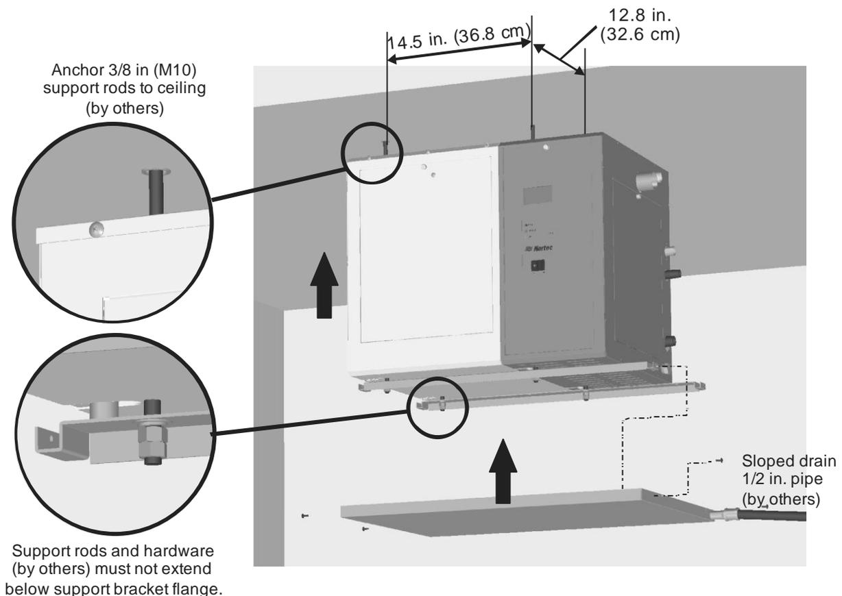
**Figure 9: Ceiling Mounting the SE50**
