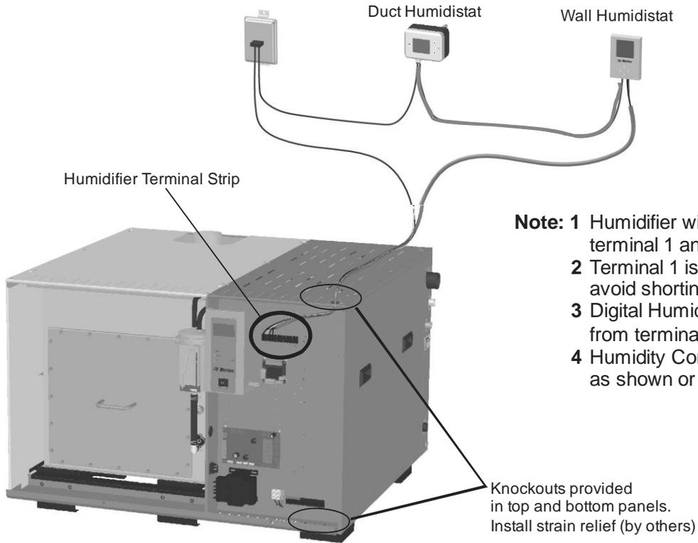
**Figure 22: On/Off Controls**
