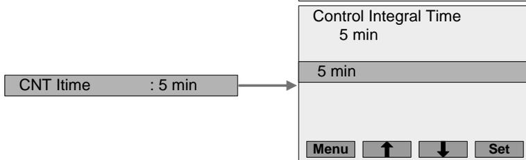
**Int Time** should not normally be changed. **Int Time** adjusts the frequency at which the controller corrects for proportional control error. It is only displayed if **REG Mode** is set to **RH (PI)** (Default = 5 min)
