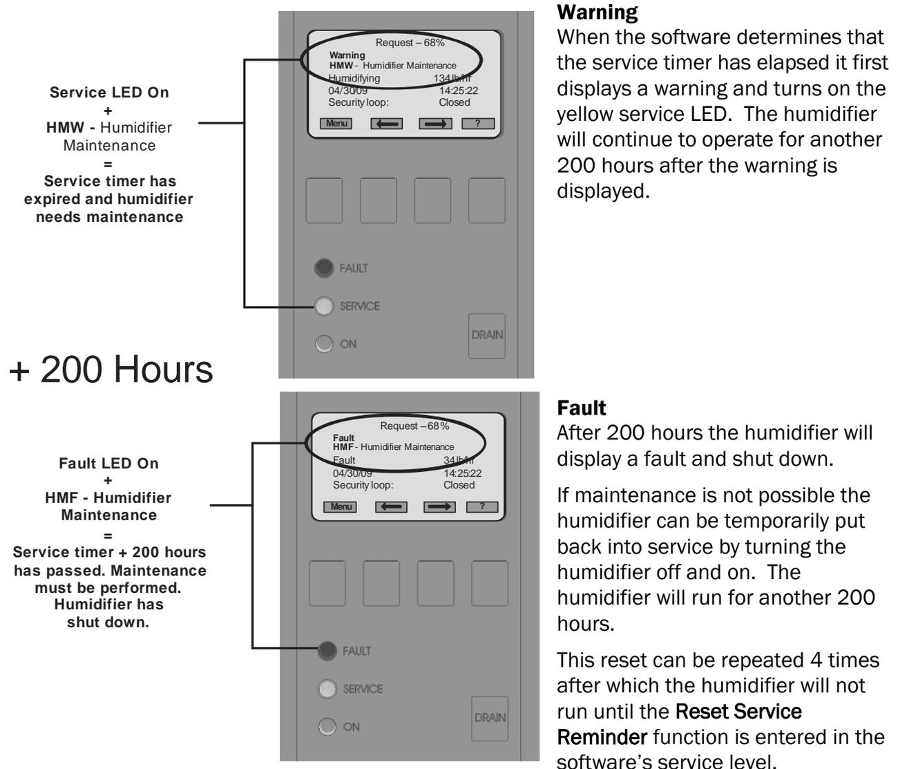
Figure 34: Service Warning / Fault
